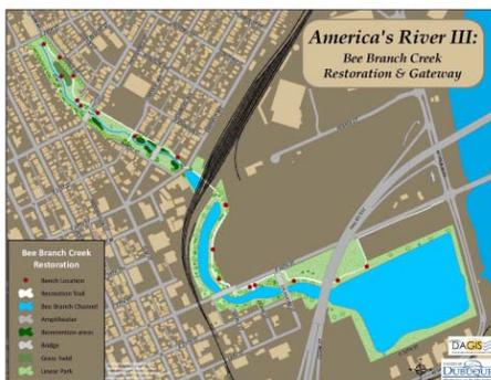
Rain events have repeatedly flooded a storm drain system known as the Bee Branch in Dubuque. Once a creek carrying runoff through the neighborhoods of Dubuque, the creek was buried 100 years ago and funneled into underground drain pipes. Now they overflow regularly. The Bee Branch restoration project is a \$61 million effort to “day-light” this former creek and create a greenway in the neighborhood. It involves voluntary buy out of 1,115 homes.
